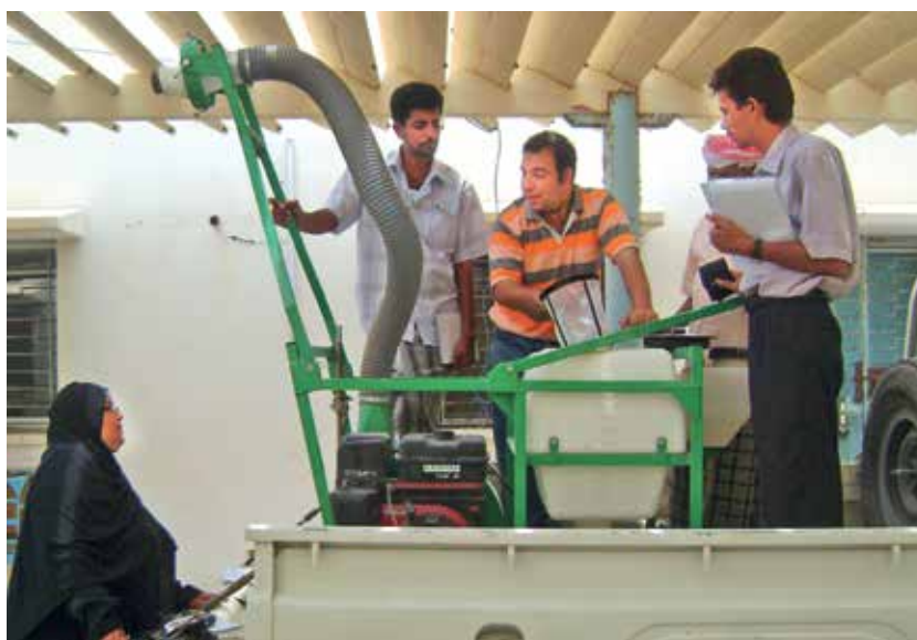
The regional master trainer from Egypt demonstrates proper calibration of a vehicle-mounted ULV sprayer during a national survey and control training course organised by the CRC in Yemen (2007)
